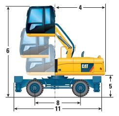
\*Dimensions with compact undercarriage, stabilizers front and rear, counterweight 4000 kg and without work tool. \*\*When the shipping height is over 4 m, the stick needs to be removed for transportation.
